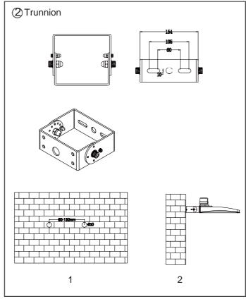
1) Drill two holes in the wall corresponding to the holes in the mounting bracket, at the position you want to install the fixture. Use expansion screws and nuts to fix the fixture tightly to the wall.
