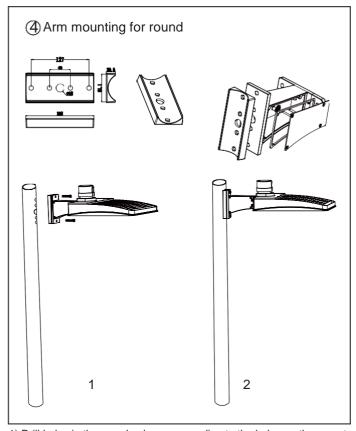
Drill holes in the round pole corresponding to the holes on the mounting arm, at the position you want to install the fixture. Use bolds and nuts to tightly fix the fixture to the pole with the adapter piece in-between.
