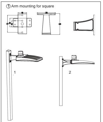
1) Drill holes in the square pole corresponding to the holes on the mounting arm, at the position you want to install the fixture. Use bolds and nuts to tightly fix the fixture to the pole.
